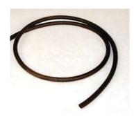
The Neoprene Tubing is industrial grade vacuum tubing that will not collapse when vacuum is applied. It is very flexible, will not crack, and stays soft. The tube has a 1/4"OD with a 1/8" ID. It can be used with 1/4" barbed fittings for easy assembly. It can be used in applications up to 200° F (93°C).
